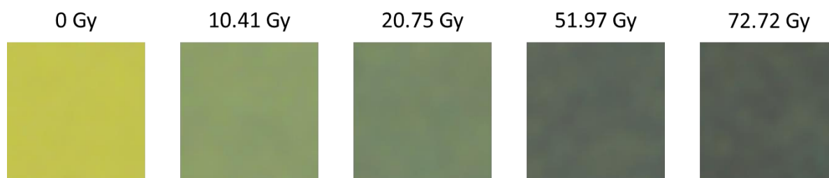
Fig. 5. Images of the dark areas of the P-EBT2 films irradiated with an alpha particle of energy 5 MeV for various doses were scanned using the Canon CanoScan flatbed scanner 9000F Mark-II with an area of 265 µm × 265 µm.
