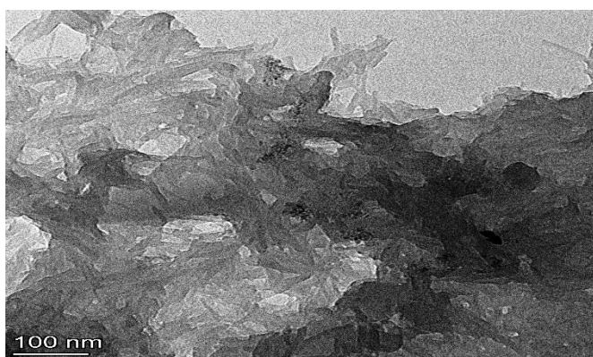
Fig.4 .The TEM image displays the dispersion pattern of the cobalt complex nanoparticles.
