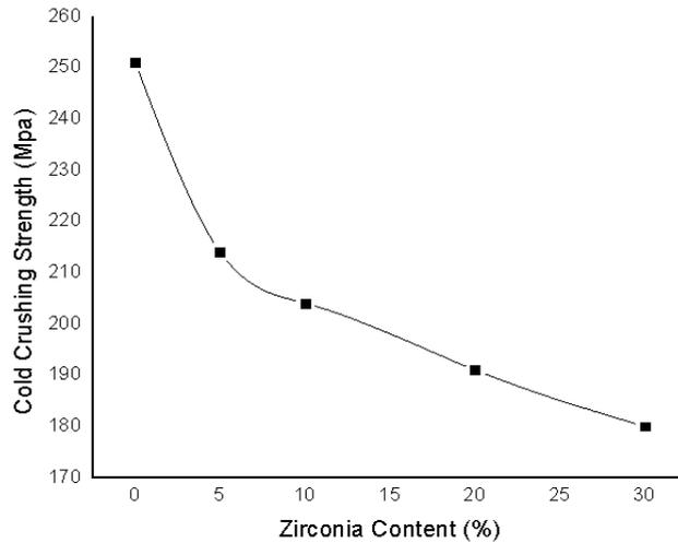
**Figure 6** Cold crushing strengths of sintered ceramic bodies.
