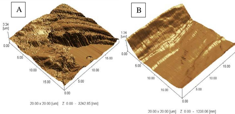
**Figure 12** 3-D image of metal cast surface poured in: (A) sand mold, (B) ceramic mold.
