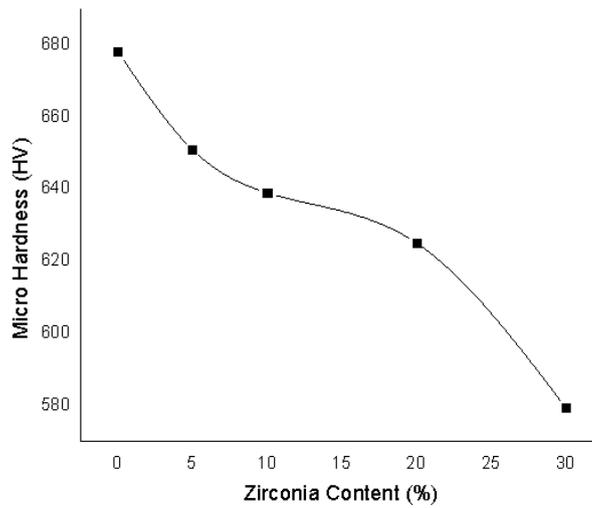
**Figure 5** Micro harnesses of sintered ceramic bodies.
