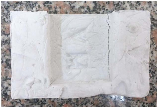
**Figure 9** Improper gelling behaviors
