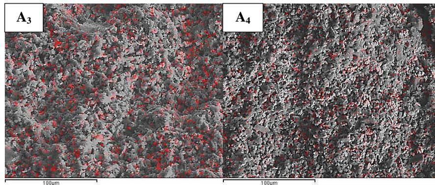
**Figure 2** Zirconia distributions in sintered ceramic bodies, where A<sub>3</sub>) 10% ZrO<sub>2</sub>, and A<sub>4</sub>) 20% ZrO<sub>2</sub> respectively.
