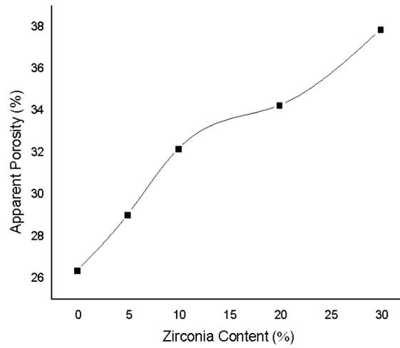
**Figure 4** Apparent porosities of sintered ceramic bodies.
