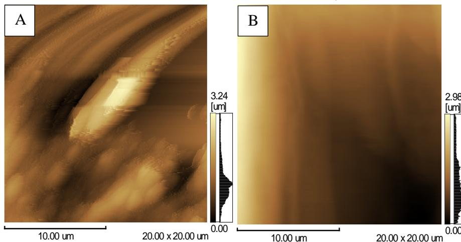
**Figure 11** Plan image of metal cast surface poured in: (A) sand mold, (B) ceramic mold.
