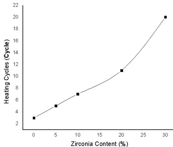
**Figure 7** Thermal shock resistances of sintered ceramic bodies
