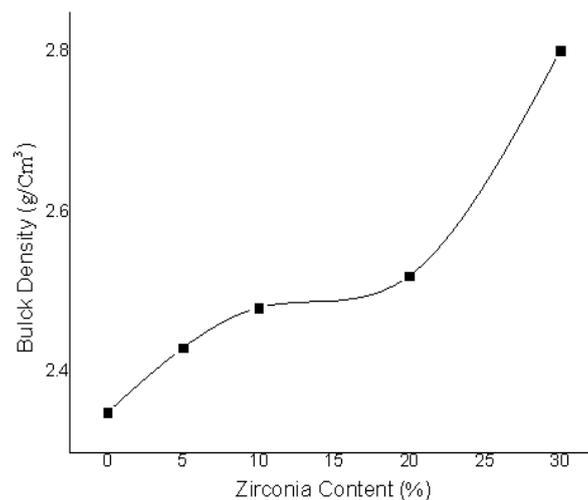
**Figure 3** Bulck densities of sintered ceramic bodies.
