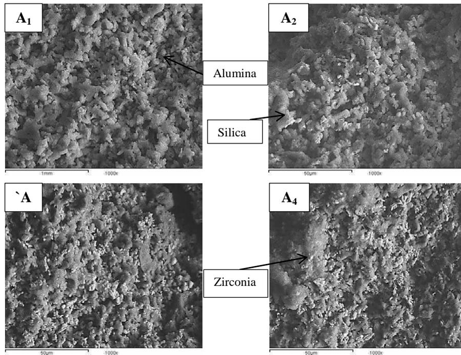
**Figure 1** (SEM) photomicrographs for sintered ceramic bodies, where A<sub>1</sub>) 0% ZrO<sub>2</sub>, A<sub>2</sub>) 5% ZrO<sub>2</sub>, A<sub>3</sub>) 10% ZrO<sub>2</sub>, A<sub>4</sub>) 20% ZrO<sub>2</sub>, and A<sub>5</sub>) 30% ZrO<sub>2</sub>
