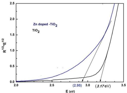
Fig.6 Band gap calculation of TiO<sub>2</sub>, TiO<sub>2</sub>/Zn respectively
