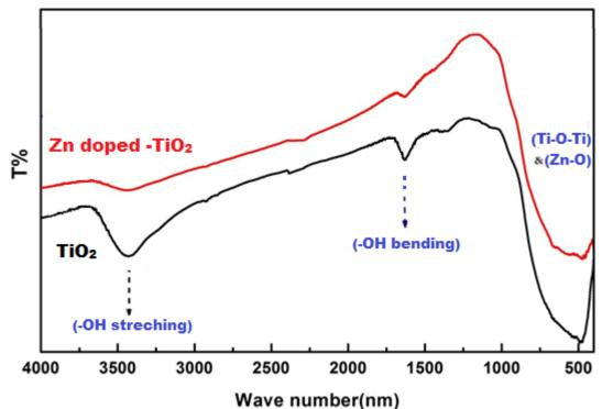
Fig.2 The FTIR curves of Zn doped -TiO<sub>2</sub>
