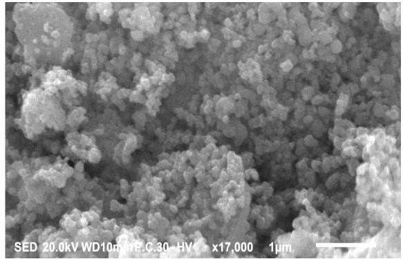
Fig.4 SEM images Zn doped -TiO<sub>2</sub> nanoparticles
