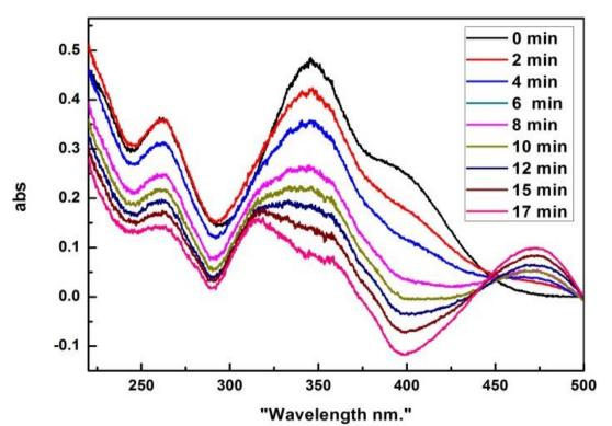
Fig.7 Efficient removal of 2, 4 dinitrophenol by Zn doped -TiO2 nanoparticles
