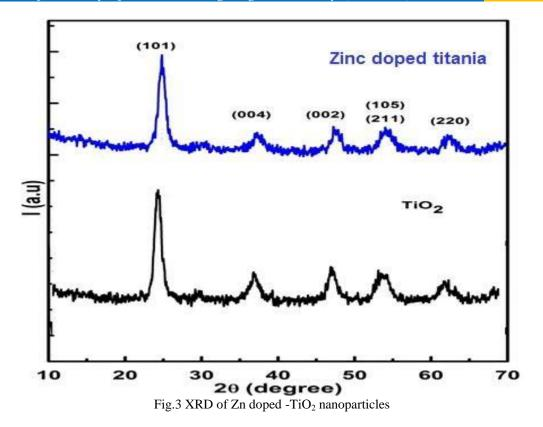
The particles sizes were found to be in the range of between 20-25 nm at the more intense x-ray beaks at  $25.2^{\circ}$ ,  $48.0^{\circ}$  and  $54.9^{\circ}$  which were smaller than that of bare TiO2(Imran, Riaz et al. 2015, Elgendy, Elmehasseb et al. 2022).
